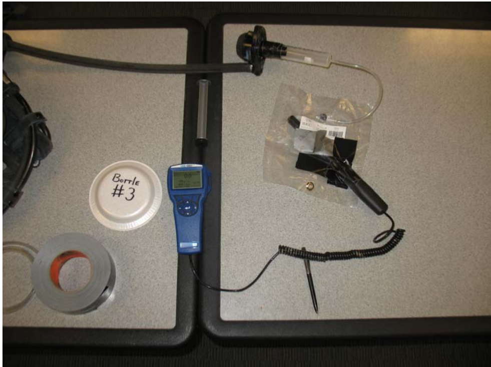
Photograph Number 1 Sampling Train Assembly
